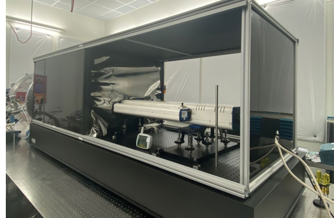
Ultra-stable lab set up with new stable composite bench and environmental enclosure.
